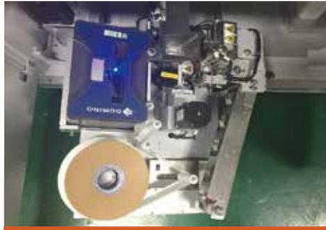
**Packaging and Printing:** The packaging unit slides out for easy replacement of packaging paper and ink bags. The sealing temperature can be adjusted. Packaging dimensions are 70\*70mm, with extended pouch lengths as needed.
