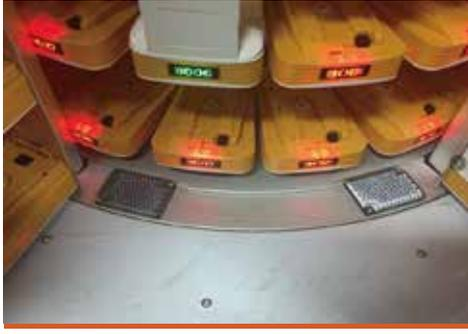
**Rotating Cabinet:** Automatically moves the medication cassette for replenishment to the medical staff by the shortest route with light prompts. It also boasts light sensors, halting rotation for safety upon detecting objects.
