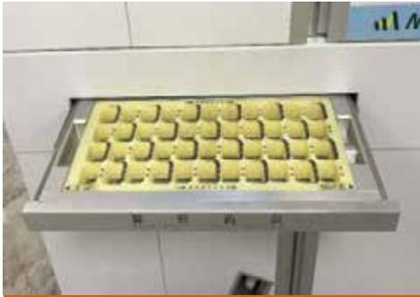
**DTA Trays:** The two trays, each with 44 compartments, are designed for half and irregularly-shaped drugs, operating alternatively to enhance efficiency. In the case of off-machine drug replenishment, the DTA trays will automatically open, with medication information provided on the screen and replenishment lists printed.
